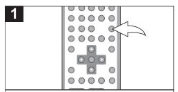
Press the P/N button to switch back and forth between NTSC and PAL. In the USA, the standard is NTSC.
